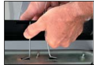
Squeeze wire-formed retainer to remove door frame.
