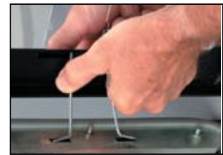
Squeeze wire-formed retainer to remove door frame.
