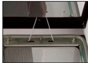
Loosen two captive, stainless steel fasteners, and door frame swings open.
